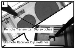
Set dip switches on the Remote Transmitter and Remote Receiver to the same settings. This must be done so the units will communcate properly. If you have other fans you can set to control from one transmitter by setting both receivers the same as the transmitter. If you have more than one fan with remote. You can set the dip switches to different positiosns to have seperate control.
