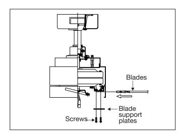
**CAUTION:** Remove the two rubber packing mounts from the fan motor assembly and discard prior to attaching the blades.
