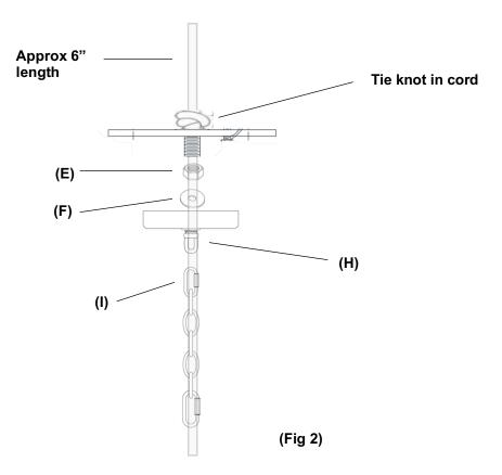
6) Re-tie the knot in the power cord, as this is for additional strain relief. Cut off the extra cord length above the knot so that it is at least 6 inches long within the outlet junction box.
