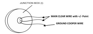
4. Insert the junction box wires through the center opening of the mounting plate (B). Attach the back plate to the wall outletbox using the two mounting screws (C) to engage with each of the back plate (B) holes.
