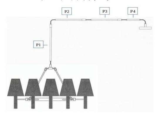
• Gently pull the slack cable out of the canopy until the assembled poles meet the thread of the Pendant Fixture (H). Screw the lower pole into the Pendant Fixture. Ensure that the poles are turned clockwise until it is secured. Hold the Pendant Fixture stationary and rotate the pole to prevent twisting of the cable.
