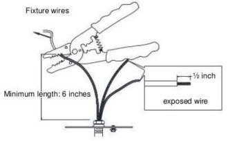
Above the canopy, measure an additional 6 inches of cord. Cut and discard any excess wire.
