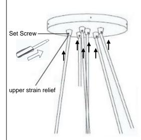
Loosen the small set screws in the upper strain reliefs using the screw driver.
