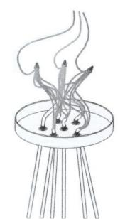
Gather all Neutral wires and twist together to prepare for connection. Gather all Hot wires and twist together to prepare for connection. Gather all Ground wires and twist together to prepare for connection.
