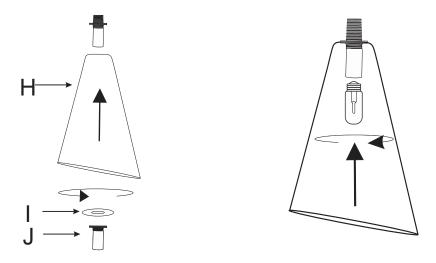
**Step 7).** Insert the Bulb (1) X 25 Watt max Type B into socket as shown in picture.
