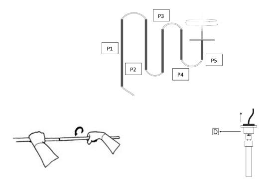
• Gently pull the slack cable through the Poles and Pipe Hook (D) until the assembled poles meet the thread of the Lamp Fixture (H). Screw the lower pole into the lamp fixture (H) by turning clockwise until fully tightened. Hold the lamp fixture stationary and rotate the pole to prevent twisting of the cable.
