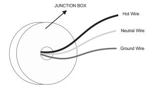
4. Insert the junction box wires through the center opening of the Mounting Plate (B). Attach the mounting plate to the wall Junction Box using the two Mounting Screws (C).
