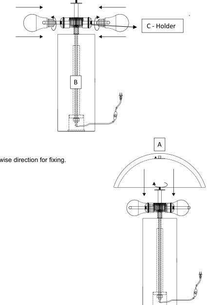
2. Place Shade on spacer and rotate shade in clockwise direction for fixing.
