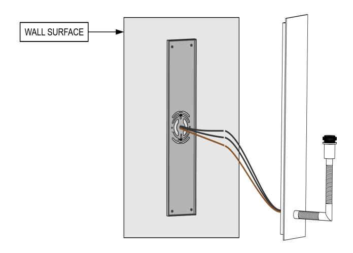
7. Place the sconce metal fixture on the mounting bracket and tighten with top screw.
