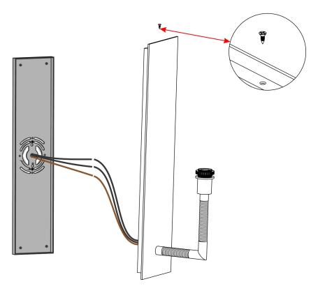
**8.** Remove the washer from the metal cap and fix the shade and tighten with washer.
