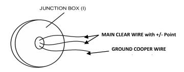
4. Insert the junction box wires through the center opening of the back plate (B). Attach the back plate to the wall outlet box using the two wall screws (C) to engage with each of the back plate (B) holes.
