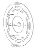
3. Gently pull existing wires out from the wall junction box and allow them to hang. The hot or live & neutral wire is clear. Check to see if there is a ground wire that is copper metal wire. If needed, use a pair of wire strippers to remove about 1/2 inch of insulation from each wire.
