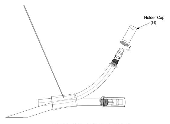
8. Fix the Glass (G1, G2, G3, G4, G5, G6, G7 & G8) onto the socket one by one and tighten the Glass by using Holder Cap (H1, H2, H3, H4, H5, H6, H7 & H8) clockwise by hand.
