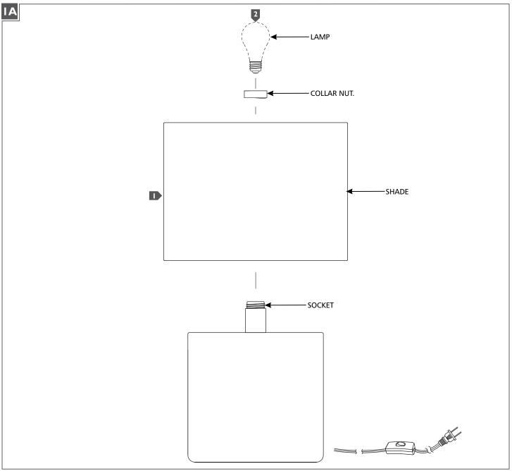
Install the shade by placing it over socket, then secure in place by screwing the collar nut onto the socket.
