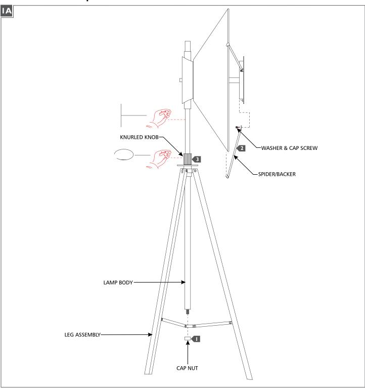
Assemble the fixture by inserting the lamp body through the leg assembly and securing in place with the cap nut.
