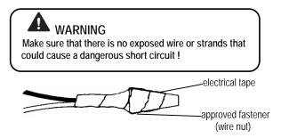
Connect the black fixture lead to the black wire in the outlet box. Fasten the joined wires as in step 4.
