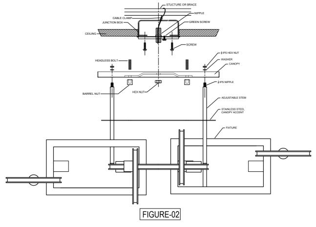
3. Place the headless bolt to the canopy that extend 3/8" beyond the canopy, then hang the fixture to the mounting strap by fastening the canopy to the nipple using hex nut. Then attach the SAFETY CABLE to the building or structure or brace. (See figure-02)
