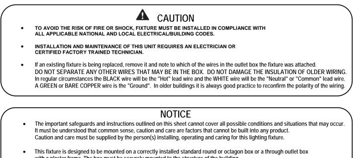
with a plaster frame. The box must be securely mounted to the structure of the building. The mounting bar and hardware supplied should be used. Directly mounting the fixture to the outlet box may make it impossible to correctly align the fixture.
