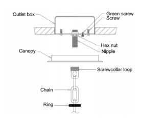
7. Open the quick links and attach the chain to the screw collar loop. Close the top link of chain.
