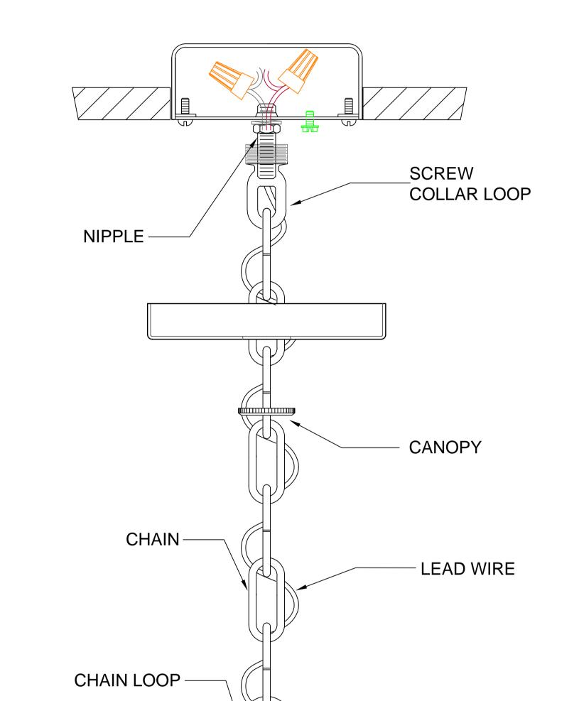
Make sure that there is no exposed wire or strands that could cause a dangerous short circuit!
