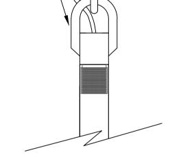
**8.** Connect the black fixture lead to the black wire in the outlet box. Fasten the joined wires as in step 7.
