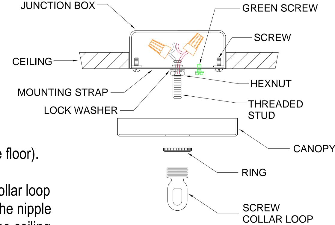
**1.** Attach the mounting strap to the outlet box. (The green screw should face the floor).
