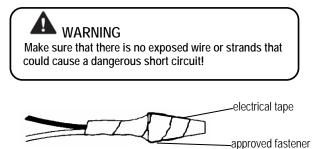
9. Connect the black fixture lead wire to the black wire in the outlet box. Fasten the joined wires as in step 8
