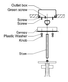
7. Fasten the ground wire to the green or bare copper wire in the outlet box or to the green screw on the crossbar.
