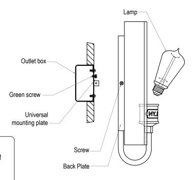
3. Fasten the white fixture lead to the white wire in the outlet box. Fasten the wires together with an approved fastener (wire nut). Starting about 1" below the fastener, tightly wrap the connection with electrical tape so that the connections seals the end of the fastener.
