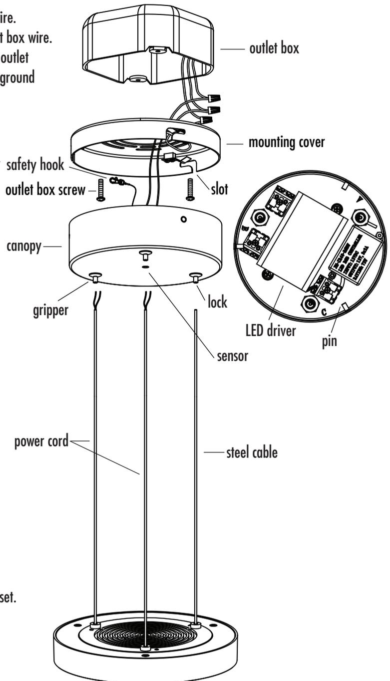
**NOTE: This fixture is controlled by the included IR remote control, which must be aimed at the sensor in the center of the canopy. The fixture may be turned on/off by a wall switch, but do not use with a wall dimmer, or damage will occur.**
