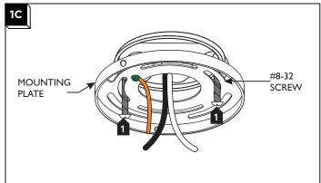
Mount the mounting plate to the electrical box with the two provided #8-32 screws.
