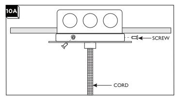
Place all wires, wire nut connections, driver properly inside the junction box.
