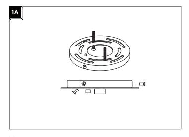
Remove the set screws from the canopy, then remove the mounting plate.
