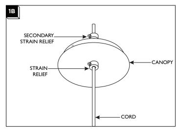
2 Feed the cord through the strain relief, canopy and secondary strain relief.
