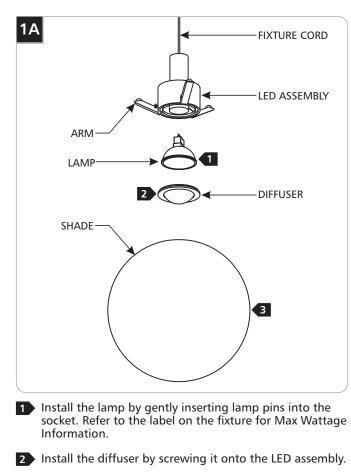
**3** Fold/hold the arms, insert the LED assembly into the shade, center the LED assembly to the shade and release the arms. Adjust as necessary.
