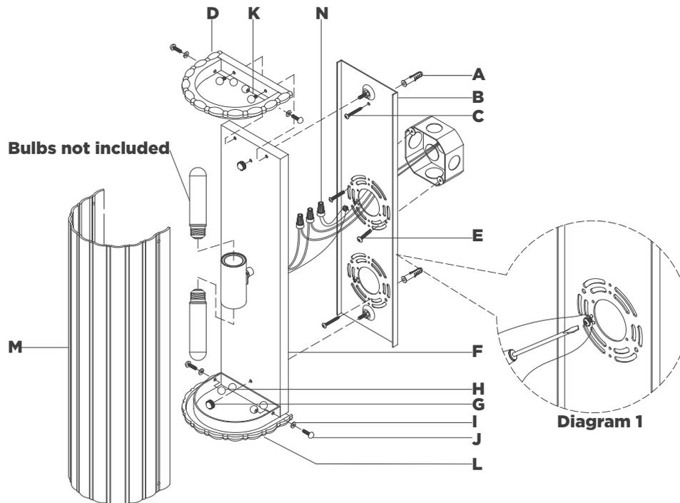
8. Connect fixture hot wire (black) to the supply hot wire (usually black) using wire nut **(N)**.
