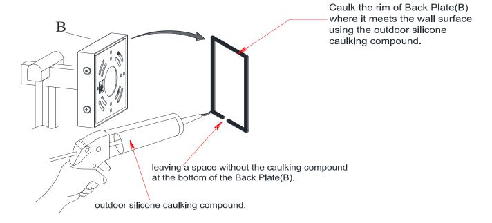
To prevent the water from entering the J-box and causing a short circuit, use the outdoor silicone caulking compound to caulk completely along the rim of Back Plate (B) where it meets the wall surface, but leaving a space without the caulking compound at the bottom of Back Plate (B).
