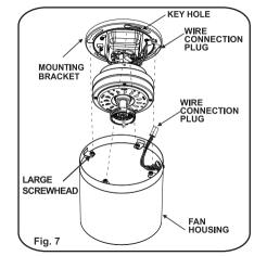
Step 2. Firmly snap the wire connection plug from fan motor assembly to the wire connection plug from fan housing. (Fig.8) Make Sure the wire connections are not in the way of the housing as you lift the housing and proceed to next step.
