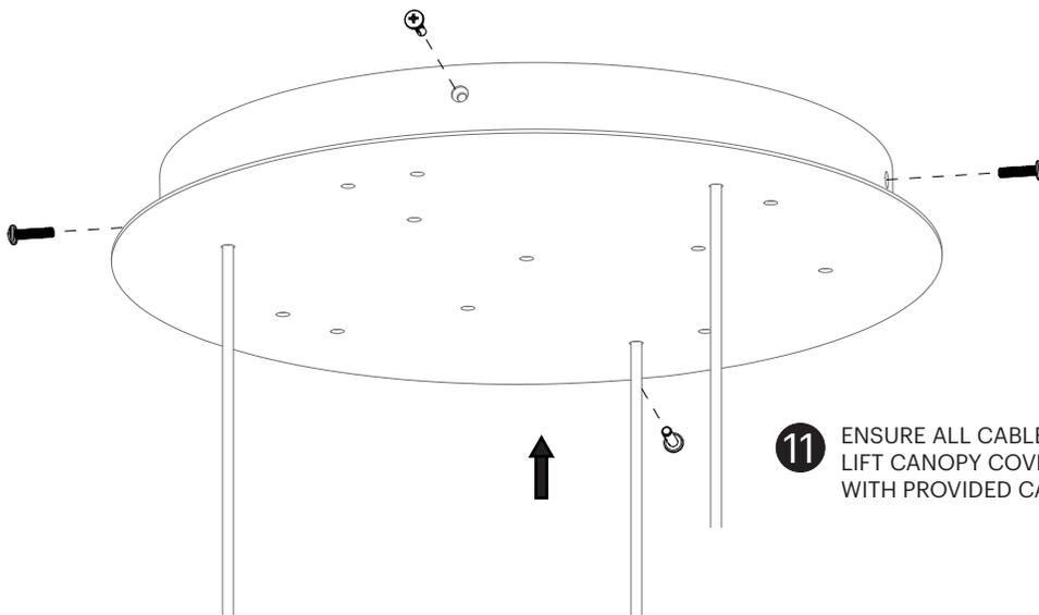
**11** ENSURE ALL CABLES AND CORDS ARE TUCKED WITHIN CANOPY COVER. LIFT CANOPY COVER UP TO CEILING AND SECURE TO MOUNTING PLATE WITH PROVIDED CANOPY COVER MACHINE SCREWS
