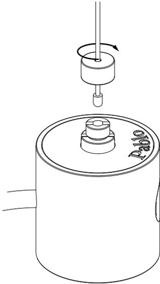
**3** THREAD CHECK RING ONTO SOCKET TO CAPTURE AND SECURE SHADE
