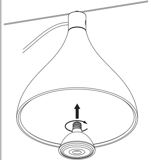
NOTE: FOR NARROW SHADE, USE PROVIDED SOCKET EXTENDER TO INSTALL BULB
