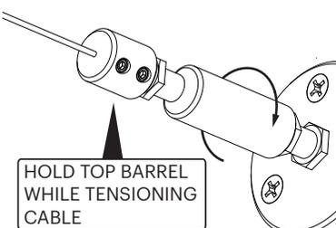
HOLD TOP BARREL WHILE TENSIONING CABLE
