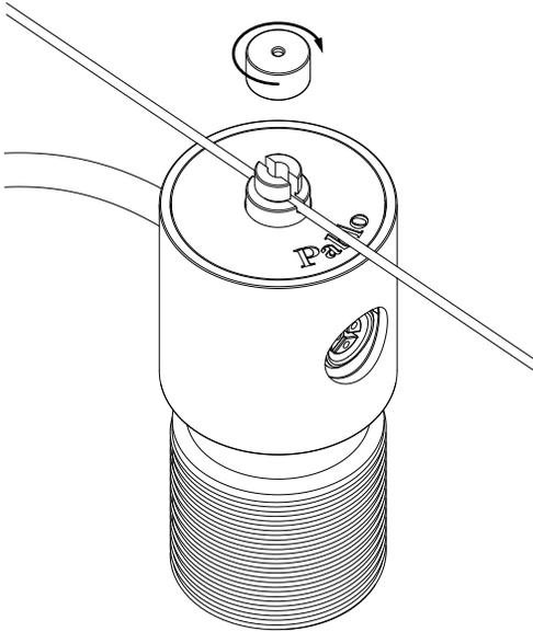
**3** THREAD CHECK RING ONTO SOCKET TO CAPTURE AND SECURE SHADE
