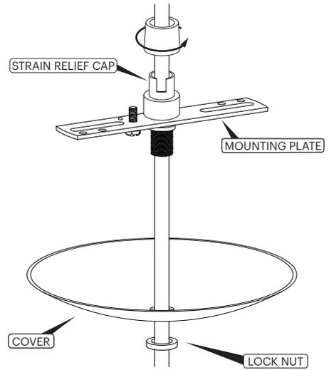
**C** TIGHTEN STRAIN RELIEF CAP AT DESIRED HEIGHT, ADDING 2-3 INCHES FOR CORD DRAPE. CUT CORD, LEAVING 6 INCHES ABOVE THE RELIEF CAP FOR WIRING
