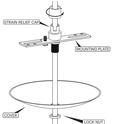
**C** TIGHTEN STRAIN RELIEF CAP AT DESIRED HEIGHT, ADDING 2-3 INCHES FOR CORD DRAPE. CUT CORD, LEAVING 6 INCHES ABOVE STRAIN RELIEF CAP FOR WIRING
