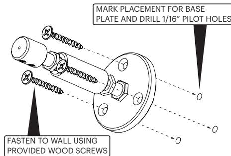
NOTE: TURNBUCKLE **MUST** BE INSTALLED ON A STUD
