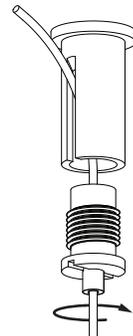
**D** DEPRESS NIPPLE ON CABLE LOCK TO ADJUST CABLE TO DESIRED LENGTH AND SCREW MALE CABLE LOCK COMPLETELY INTO FEMALE CABLE LOCK MOUNT TO FINISH INSTALLATION
