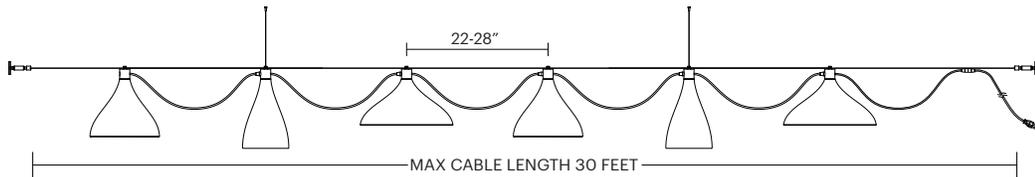
**WARNING: MAXIMUM OF 34 INTERCONNECTED 14.5W LAMPS, DO NOT EXCEED 500 TOTAL WATTS**
