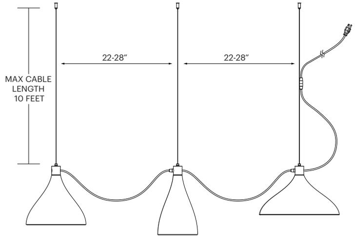
**WARNING: MAXIMUM OF 34 INTERCONNECTED 14.5W LAMPS, DO NOT EXCEED 500 TOTAL WATTS**
