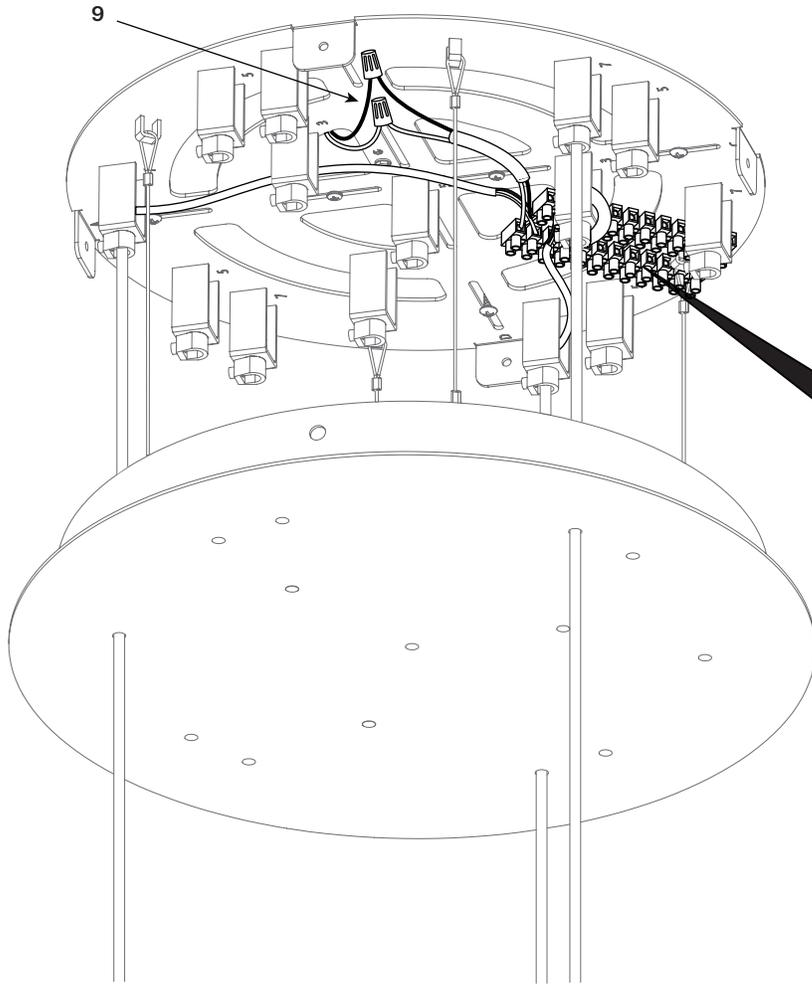
**9** CUT CORDS TO REACH 12-PORT TERMINAL BLOCKS, ALLOWING FOR 3" OF EXTRA CORD PAST TERMINAL BLOCKS. STRIP CORDS SO LEAD WIRES ARE EXPOSED, THEN WIRE CORDS TO TERMINAL BLOCKS AS SHOWN AND SECURE WITH #2 FLAT HEAD SCREW DRIVER
