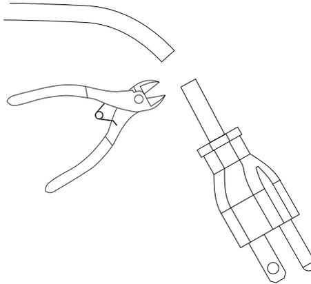
**B** LOOSEN STRAIN RELIEF CAP AND FEED CORD THROUGH ALL COMPONENTS
