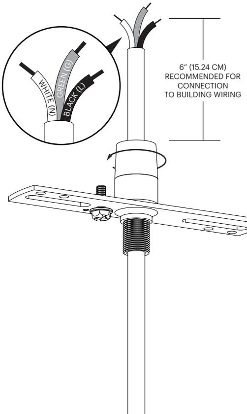
**D** ATTACH MOUNTING PLATE TO JUNCTION BOX, CONNECT BUILDING WIRING TO FIXTURE WIRING. CONNECT FIXTURE GROUND WIRE TO AND BUILDING GROUND WIRE TO GREEN GROUND SCREW ON MOUNTING PLATE. SLIDE CANOPY COVER UP TO CEILING, THEN SECURE COVER TO PLATE WITH THE LOCK NUT
