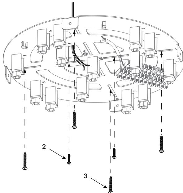
**2** ATTACH PLATE TO JUNCTION BOX WITH PROVIDED JUNCTION BOX MACHINE SCREWS
