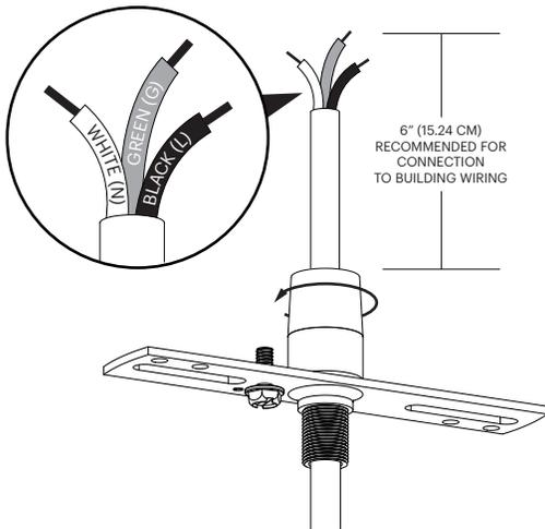
**D** ATTACH MOUNTING PLATE TO JUNCTION BOX, CONNECT BUILDING WIRING TO FIXTURE WIRING. CONNECT FIXTURE GROUND WIRE TO AND BUILDING GROUND WIRE TO GREEN GROUND SCREW ON MOUNTING PLATE
