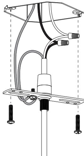
**E** SLIDE COVER UP TO CEILING, THEN SECURE COVER TO PLATE WITH THE LOCK NUT
