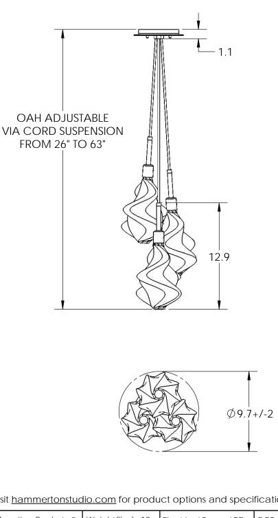
\*\*NOTE\*\* DRIVER TO BE INSTALLED IN J-BOX MINIMUM SIZE OF J-BOX REQUIRED IS 4" L x 4" W x 1.5" H
