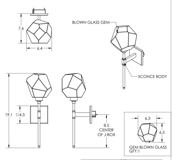
\*\*NOTE\*\* DRIVER TO BE INSTALLED IN JUNCTION BOX. MINIMUM SIZE J-BOX REQUIRED IS 4" L X 4" W X 1.5" D
