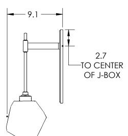
\*\*NOTE\*\* DRIVER TO BE INSTALLED IN JUNCTION BOX. MINIMUM SIZE J-BOX REQUIRED IS 4" L X 4" W X 1.5" D
