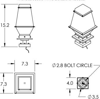
Mounting Method: Mounts Directly To Pier
