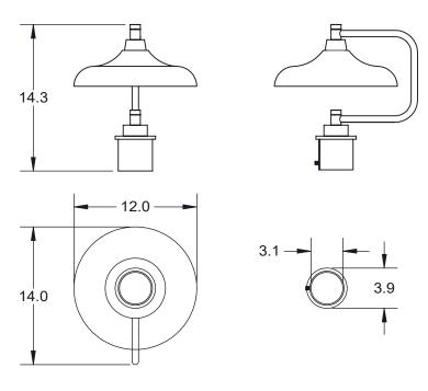
Mounting Method: Mounts Directly to Post
