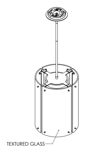
\*\* NOTE\*\* DRIVER TO BE INSTALLED IN J-BOX. MINIMUM SIZE OF J-BOX REQUIRED IS 4" L x 4" W x 1.5" H
