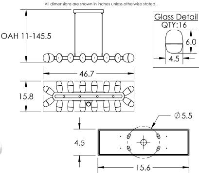
Mounting Method: Mounts to Building Structure
