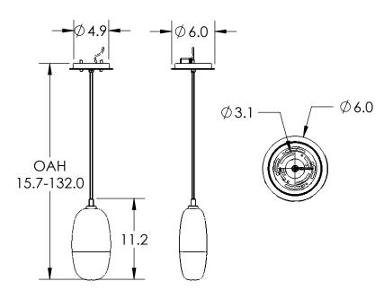
Mounting Method: J-Box Ceiling Mount. Minimun J-Box Size Requirement is 4" W, 4" L, 1.5" D
