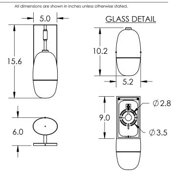
Mounting Method: J-Box Wall Mount. Minimum J-Box Size Requirement is 4" W, 4" L, 1.5" D
