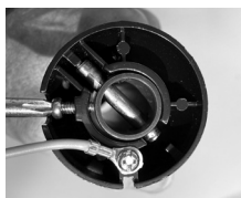
remove half-ball and stopper pin
