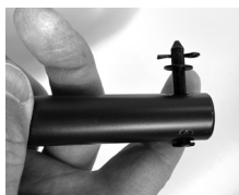
remove stopper pin, cotter pin and washer
