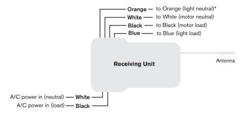
\* If fan does not have orange wire, cap orange wire from receiving unit.
