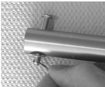
remove stopper pin, cotter pin and washer
