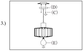
Step3: Install fixture to bracket and tighten screws at the ends of the canopy to secure. Install bulb into Socket.
