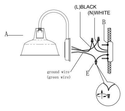
$2.\,$  Caulk around backplate where fixture meets the wall leave a hole at the bottom to allow water to escape.
