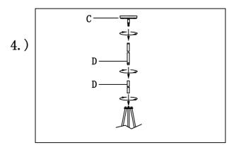
Step. 4: Run wire through stems (D) and combine stem lengths to meet desired mounting height.
