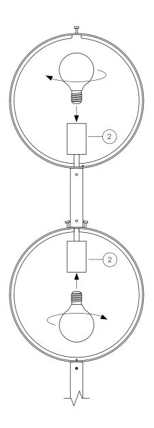
Insert the glass parts ③ into the hoops ④. At the upper hoop the groove in the glass ⑤ must fit the tube ⑥. The glass edges at the bottom of the mounting hoop must fit behind the pins ⑦.
