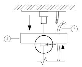
Install the wiring. Then affix the canopy (4) to the mounting plate (1) as in step 3. The power supply cable should twist at least once around the load-bearing cable as shown in the diagram below.
