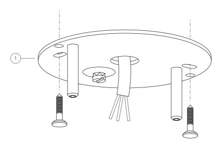
Loosen the grommet  $\ensuremath{ \mathfrak{I}}$  and slide the cable  $\ensuremath{ \mathfrak{B}}$  through the canopy  $\ensuremath{ \mathfrak{Q}}.$
