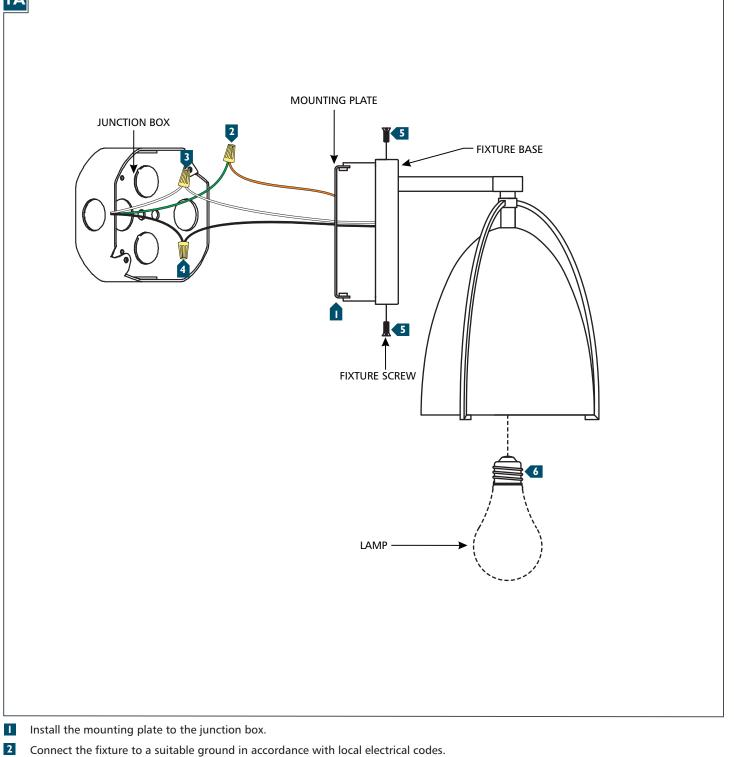
Connect the white fixture wire (square and/or rigid) to the neutral power line wire with a wire nut.
