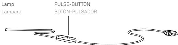
**ON/OFF:** Quick pulse (less than 1 sec.)
