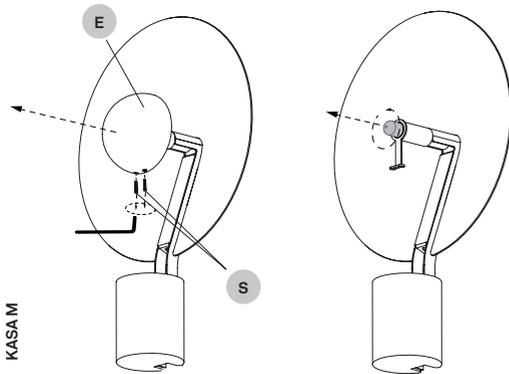
In order to change the bulb in KASA M, first remove the semispherical reflector (E) using an allen key to undo the screws (S). Then you will be able to access the bulb to change it.
