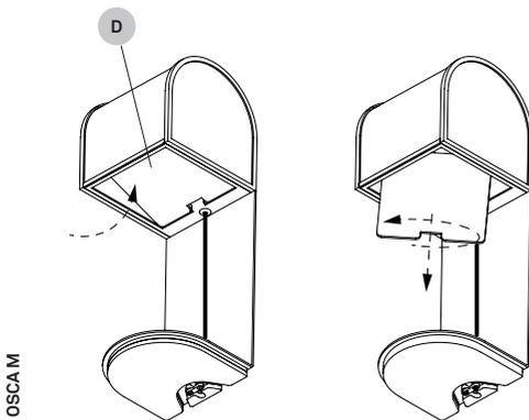
In order to change the bulb in OSCA M, first remove the acrylic diffuser (D) by pushing in inside the shade. This piece is attached by magnets.
