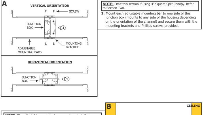
**NOTE:** The adjustable mounting bars mount to stude that are spaced 15"-24" apart. If the span needs to be shorter than 15", then break the bar arms from dedicated lines.
